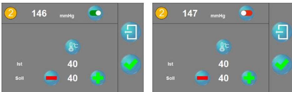
The deactivated sensors are indicated by "hyphens" in the ***initial display***. This setting is not possible during an ongoing measurement.
