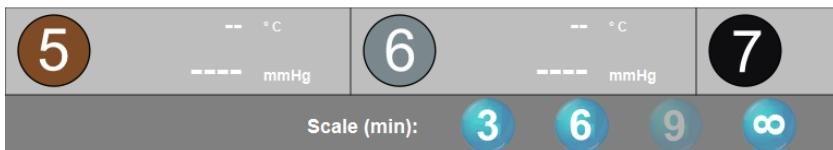
By selecting the scaling between 3, 6 or 9 minutes, the last minutes of the measurement graph of a live measurement can be shown on the display.
