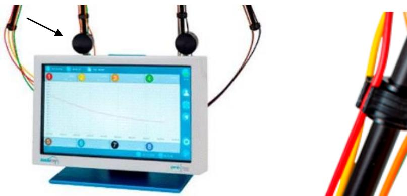
Carefully insert the optical fibre cable into the guide clips.
