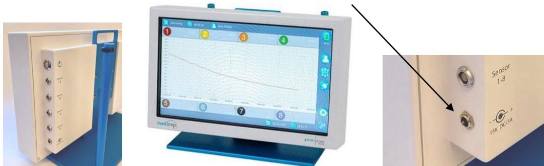
Plug the power supply into the contact socket (100 to 240 VAC).
