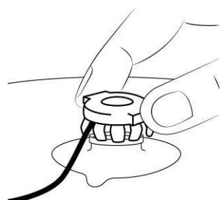
The sensor head can be inserted into the adhesive ring using a one-touch click system. To prevent the sensor from shearing off, ensure that there is no tension on the cable when inserting it.
