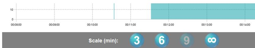
By selecting the scaling between 3, 6 or 9 minutes, the last minutes of the measurement graph of a live measurement can be shown on the display.
