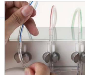
Colour coded tube system: facilitates equipping and prevents confusion
