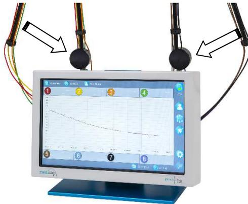
Carefully insert the optical fibre cable into the guide clips.
