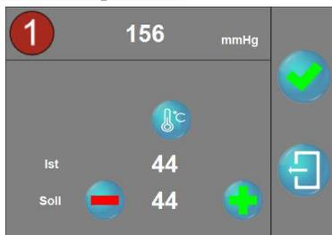
In the menu item “Parameters”, the target temperature can be changed by pressing the
