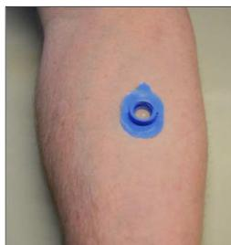
Use only **ONE-TWO drops** of contact fluid into fixation adhesive ring (as large as a pinhead). The probe can be fixated by **rotation in clockwise** direction using the thread on the fixation adhesive ring – approx.  $\frac{1}{2}$  turn. Note that, during this fixation rotation, no pulling tension is caused at the cable.
