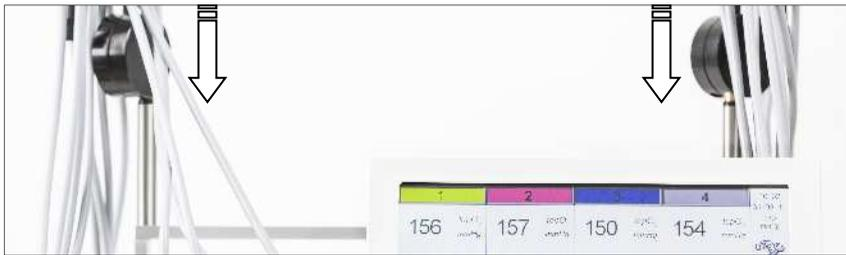
Insert the optical fibres cables carefully into the routing clips
