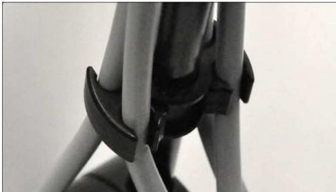
**Attention:** Do not bend or fold the optical fibres cables around the joints. The optical fibres cables need space when assorting them to avoid cable breaks.
